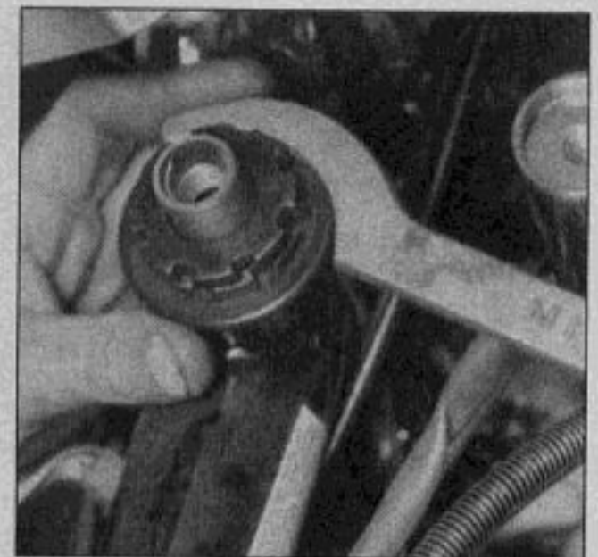
25.8 Use a spanner wrench like this one to loosen or tighten the steering stem locknuts (upper triple clamp removed for clarity)
