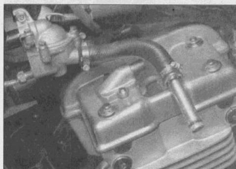
9.3 Pull the tubes out of the cylinder head and remove the O-rings with a pointed tool
