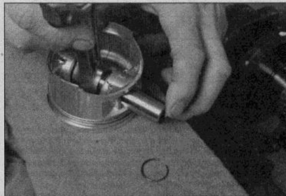
14.15 Slip the pin into the piston and try to wiggle it back-and-forth; if it's loose, replace the piston and pin
