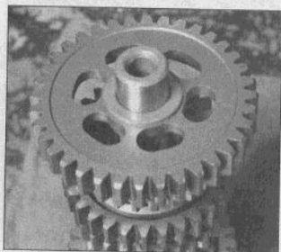
30.17l Install first gear and its spacer...
