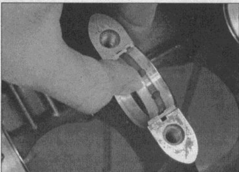
25.7 To remove a main bearing insert, push it sideways and lift it out
