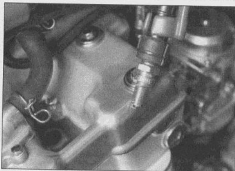
2.3 With the wire attached, ground (earth) a spark plug to the engine and operate the starter - bright blue sparks should be visible
