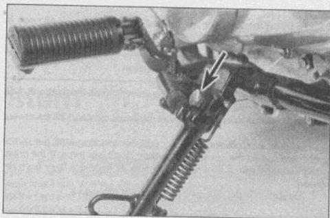
4.3 With the motorcycle securely supported, unhook the spring and remove the pivot bolt (arrow) to detach the sidestand
