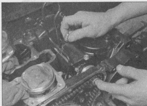
26.7 Lift the starter and disengage it from the chain
