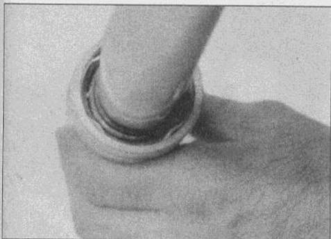
4.21 Install the retaining ring and make sure it seats in its groove
