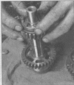
30.15k ...and slide sixth gear off the shaft
