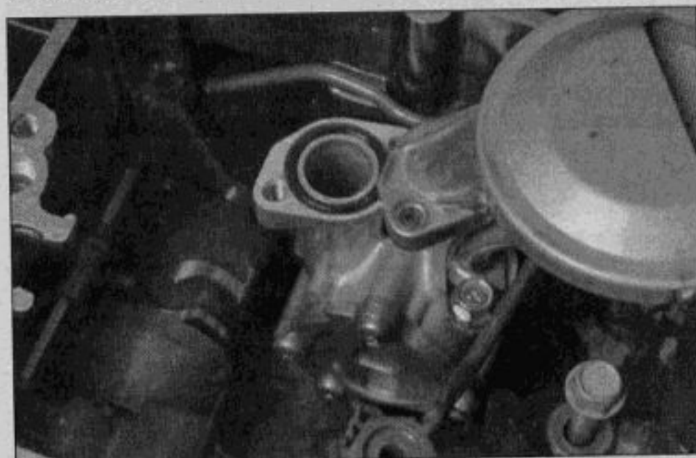
17.8 Unbolt the pickup from the pump so you can inspect the O-ring - use non-permanent thread locking agent on the bolt threads during assembly
