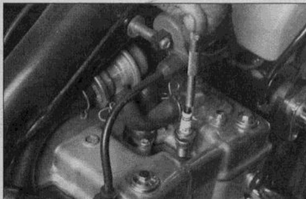
15.2c Use an extension and a deep socket (preferably one with a rubber insert to prevent damage to the plug) to remove the spark plugs; a magnet can be used to lift the plugs out of the head once they're loose
