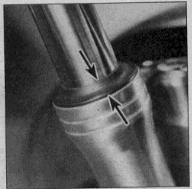
28.3 Check above and below the fork seals (arrows) for signs of oil leakage
