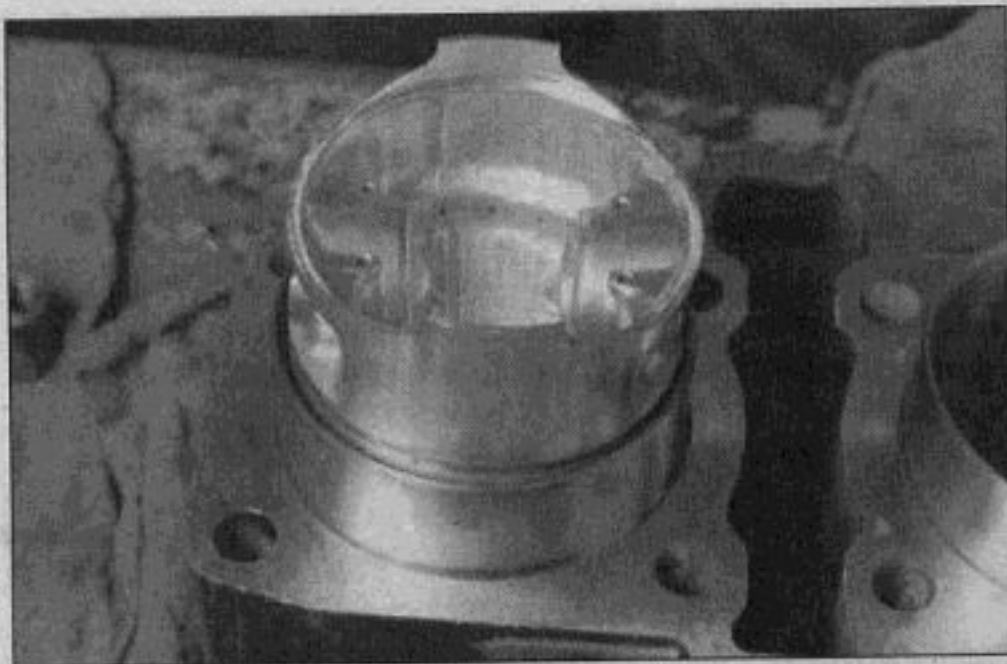
15.3a Square the ring in the bore by turning the piston upside down and tapping on the ring. . .
