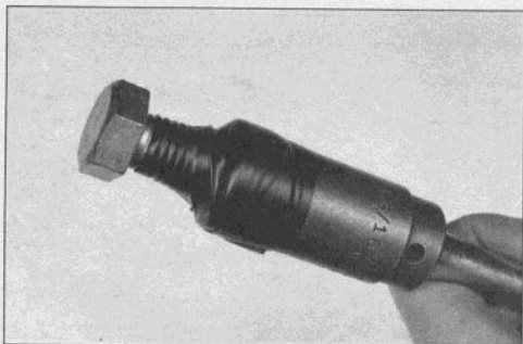
4.4d . . . then install the nut-end into a socket (connected to a long extension) and tape it into place
