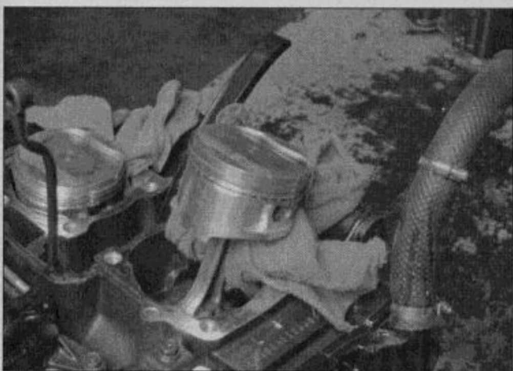
13.6 Place rags under the pistons to protect them and keep debris out of the crankcase
