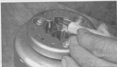
35.4a Compress the springs with a small screwdriver and remove the rollers
