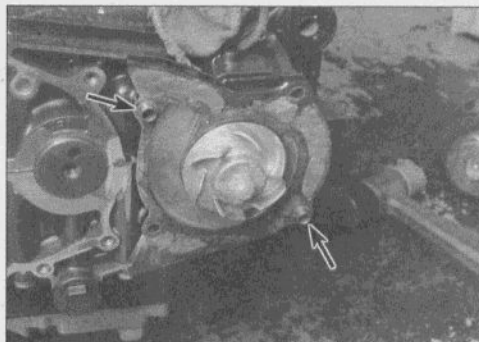
8.18 Position the housing on the engine, install a new gasket and the dowels (arrows); turn the impeller counterclockwise (anticlockwise) to install it on the shaft
