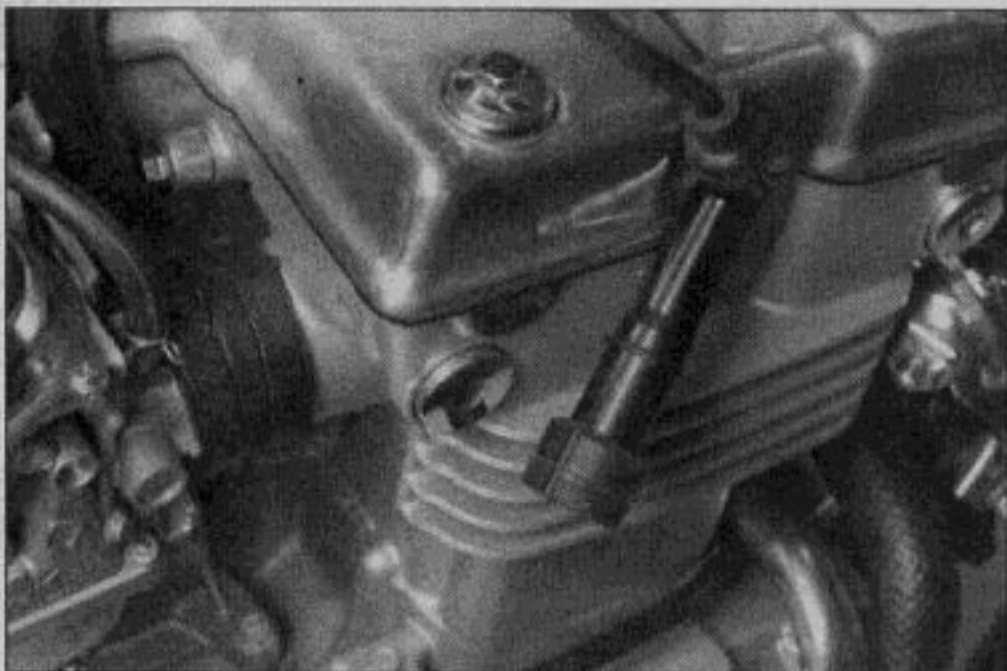
15.2b . . . then pull them off the plugs and check them for brittleness and cracking
