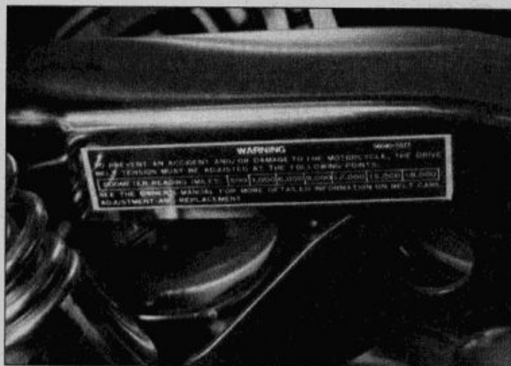
2.3c A decal on the drive belt guard lists belt maintenance intervals
