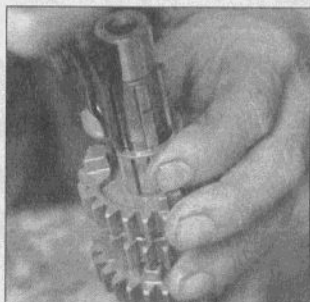
30.4f . . . then remove the snap-ring. . .
