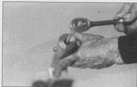
4.4b Hold the damper rod and remove the screw with an Allen wrench
