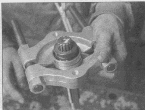
30.15p If the bearing is worn or damaged, place it in a bearing splitter, press it off the shaft and press a new one on (or have the job done by a motorcycle dealer)
