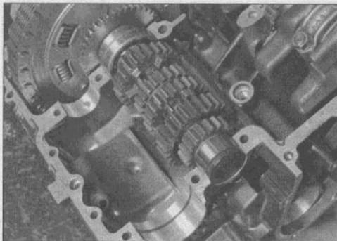
29.3b ...the main drive shaft is removed together with the clutch housing
