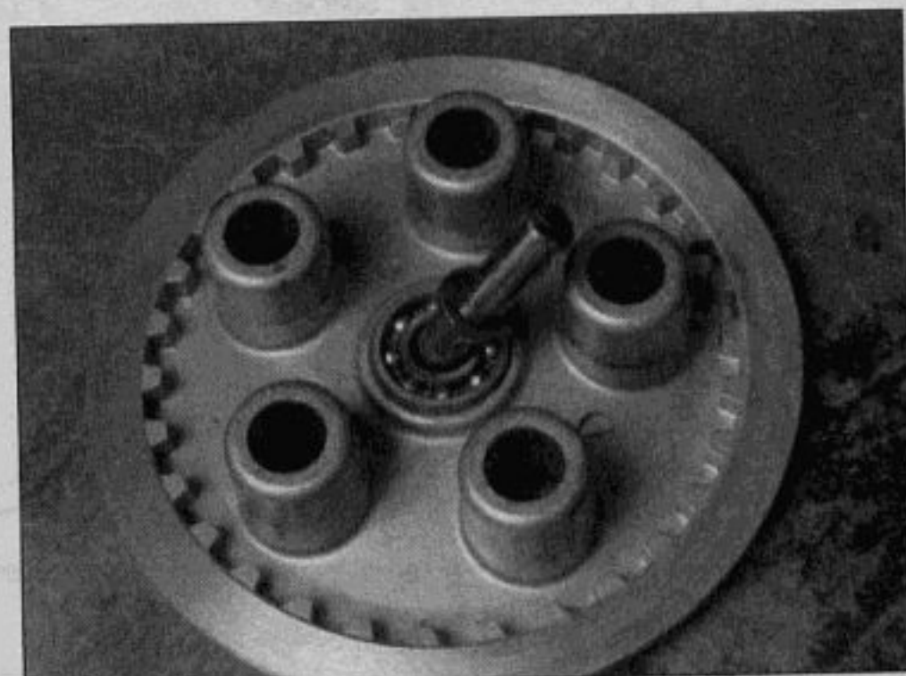
19.16 Check the pushrod and the bearing in the spring plate for wear and damage
