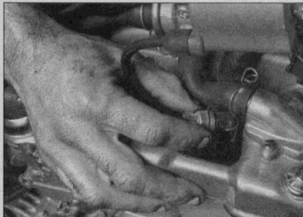
15.2a Rotate the spark plug caps back and forth to loosen them . . .
