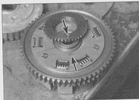
25.30a The pin in the oil pump drive gear must engage the notch in the clutch housing (arrows) . . .
