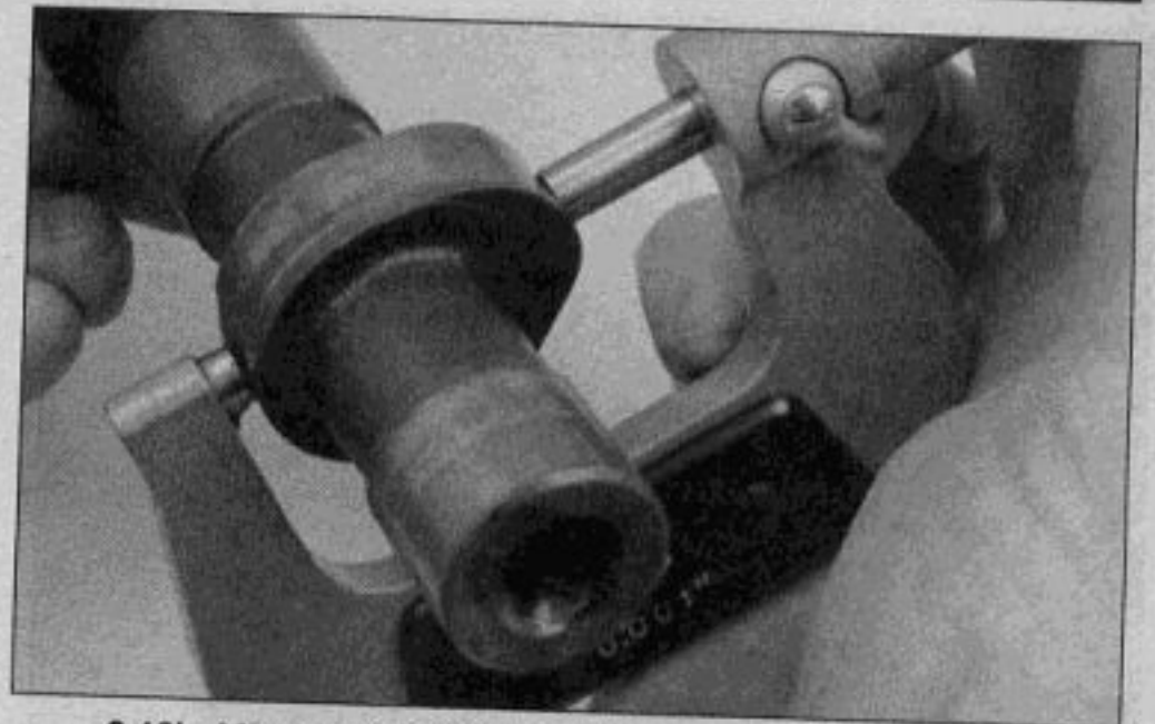
9.10b Measure the height of the camshaft lobes with a micrometer
