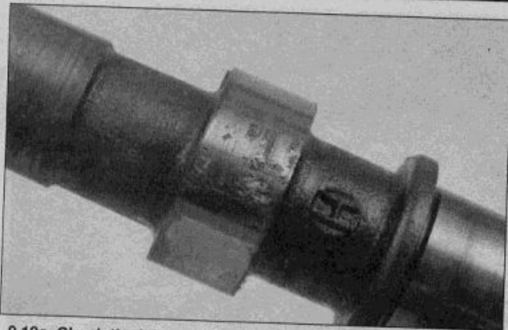
9.10a Check the lobes of the camshaft for wear - here's a good example of damage which will require replacement (or repair) of the camshaft
