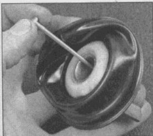
7.5b Remove the needle from the piston
