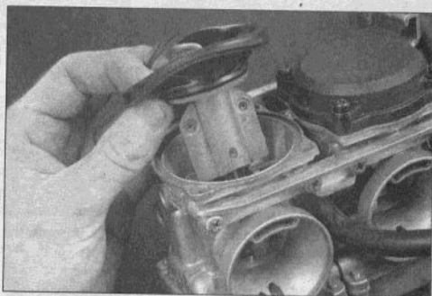
7.4 Remove the diaphragm/piston assembly from the carburetor body
