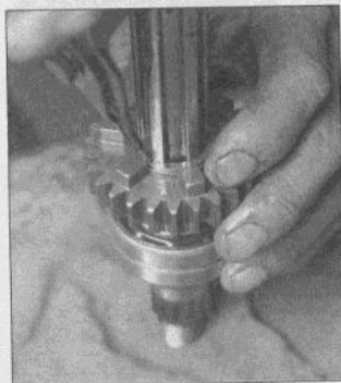
30.4h ...remove the snap-ring and toothed washer...
