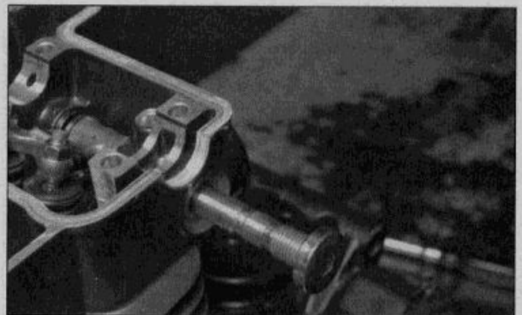
9.30b . . .unscrew the shaft and pull it out
