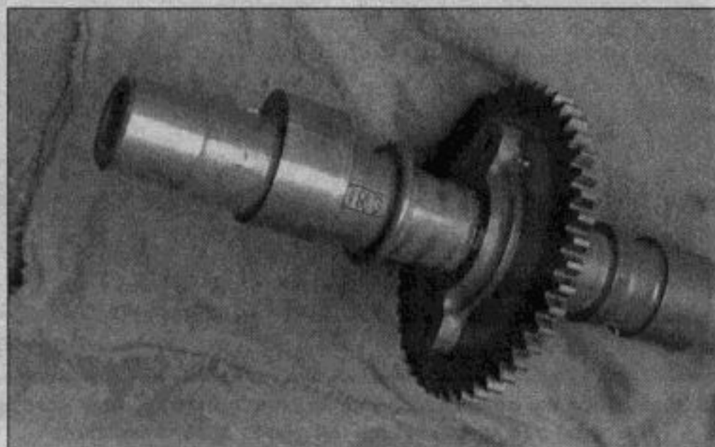
9.7b The camshafts are identified by punch marks
