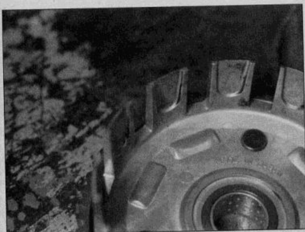
19.15 Check the slots on the clutch housing for indentations - if they're worn, the crankcase will have to be disassembled to remove the clutch housing
