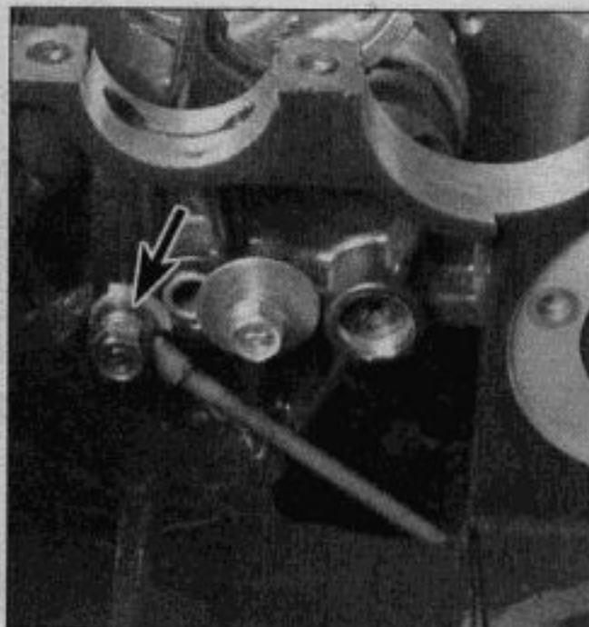
22.9b Remove the main oil pipe connecting bolt on the side of the case (arrow) . . .
