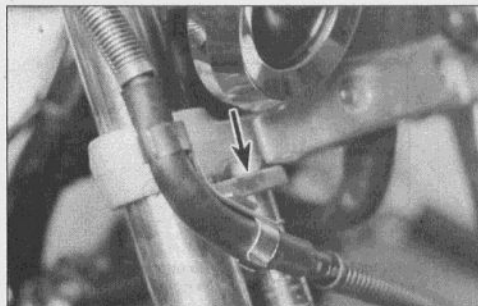
7.3 Unbolt the hose bracket from the lower triple clamp (arrow)
