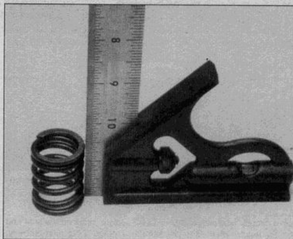
12.19b Check the valve springs for squareness
