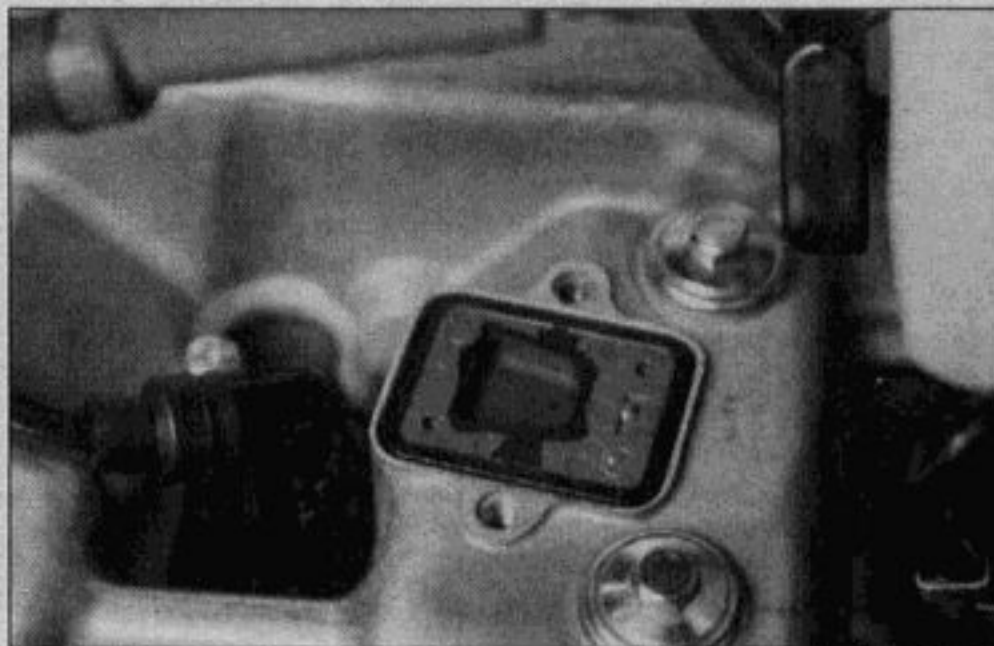
23.3b Unbolt the air suction valve from the valve cover to inspect it
