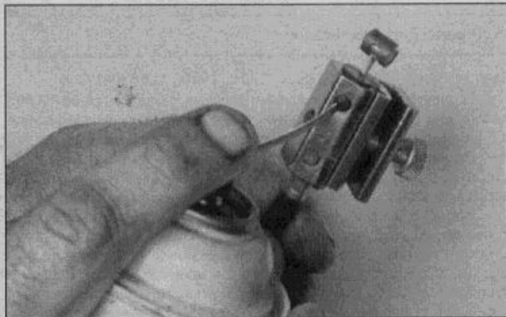
16.3b Lubricating a cable with a pressure lube adapter (make sure the tool seats around the inner cable)
