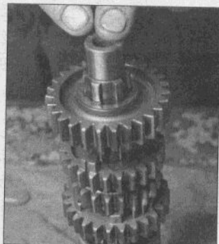
30.11g Install sixth gear with its flat side away from fourth gear and place a toothed washer next to it...
