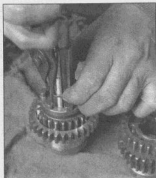
30.15j Remove the toothed washer, then the snap-ring...
