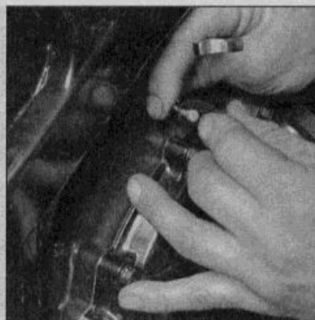
19.4 Disengage the end of the cable from the release lever
